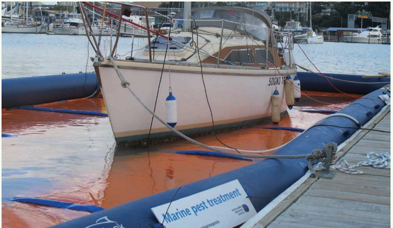
Inflatable vessel quarantine facilities, such as the one shown in use at Westhaven, Auckland, can be used to treat the infected hulls of vessels in a variety of locations (Northland Regional Council)
